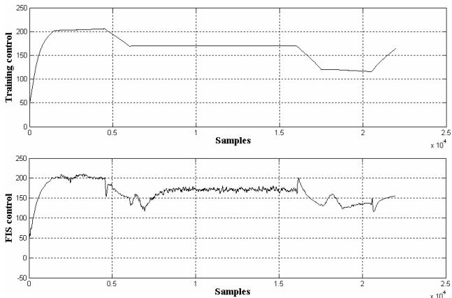
Figures 4: The training control / the speed NFC output for selected and filetered data: 22001 data, 100 epochs.
