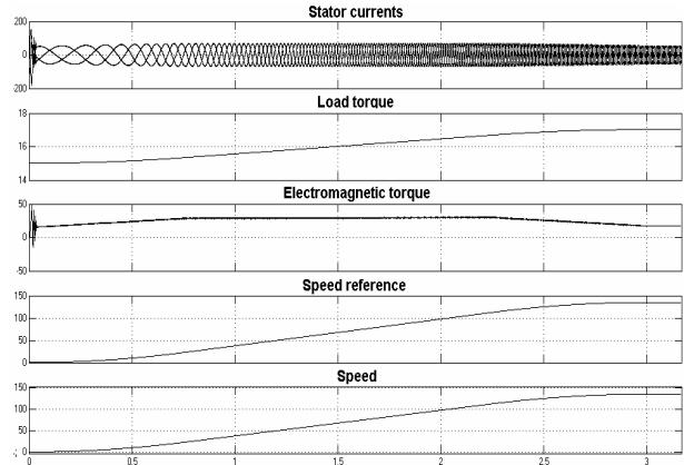
Figures 11: The results for a system with an optimized DISO speed NFC and SISO current NFCs (no shock operation).
