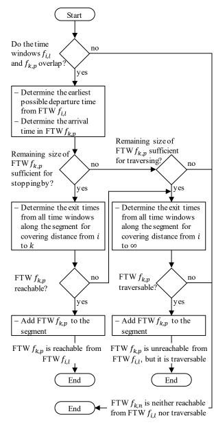
Figure 7: Reachability check of free time window  $f_{k,p}$
