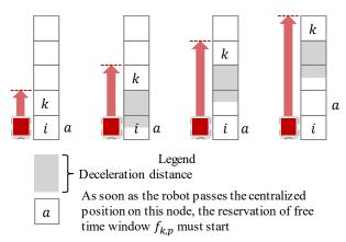
Figure 12: Determination of the start of the reservation of the free time-window  $f_{k,p}$
