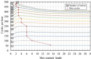
Figure 15: Throughput using the triangle reservation mechanism
