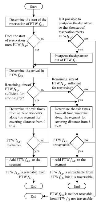
Figure 14: Reachability check of free time window  $f_{k,p}$
