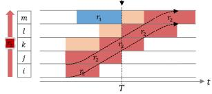
Figure 13: Robot  $r_1$  being late leads to an unplanned intermediate stop on node l for robot  $r_2$ .
